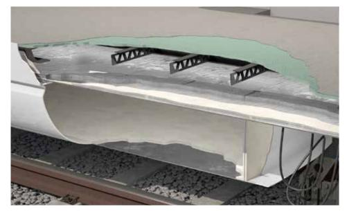
To prevent condensation in floor constructions our closed-cell ArmaFlex Rail forms a reliable vapour barrier and mitigates the risk of corrosion.
