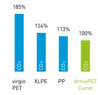
CO2 emissions of ArmaPET products in comparison to competitive materials. ArmaPET = 100% reference
