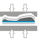
Picture 2: Cold mould press
